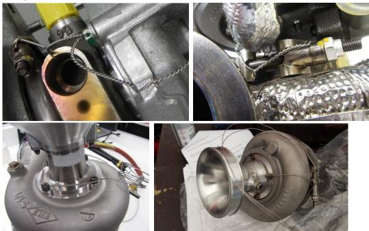
Examples of incorrect sealing wiring
